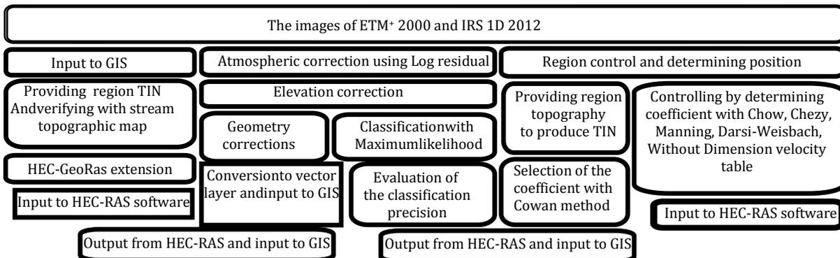
Fig.3. All of the stages and the method of determining of land use and flood plain
