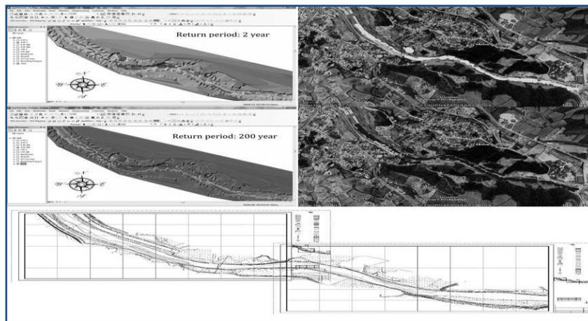
Fig.5. Cross and longitudinal sections and The flood zone in return periods of 2 and 200 year
