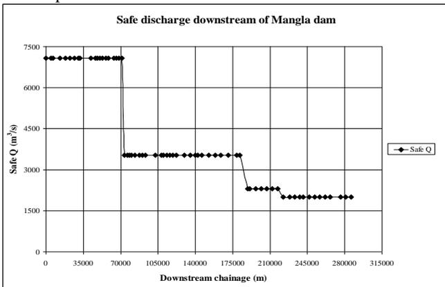
Fig. 4. Safe discharge downstream of Mangla dam
