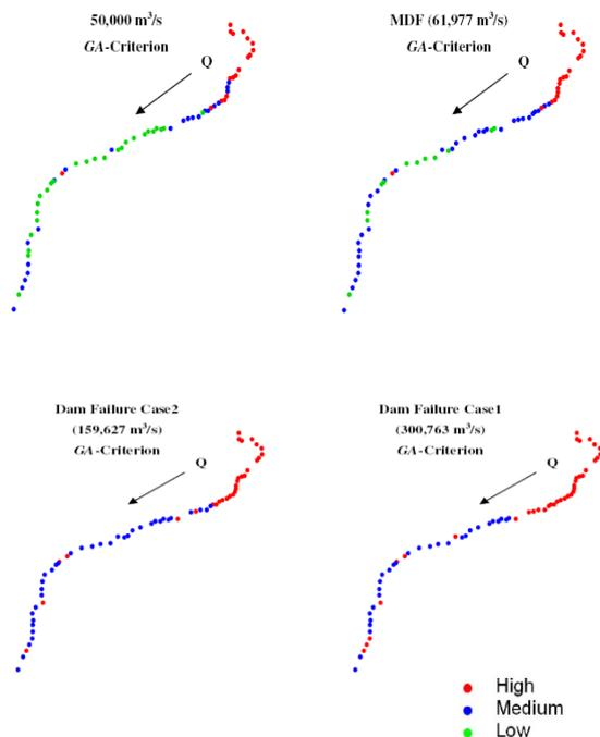
Fig. 8. Flood severity downstream of Mangla dam
