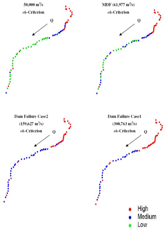
Fig. 6. Flood severity downstream of Mangla dam ( $vh$ -criterion: with bridges)
