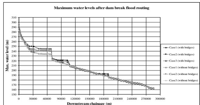
Fig. 3. Maximum water levels after dam break flood routing
