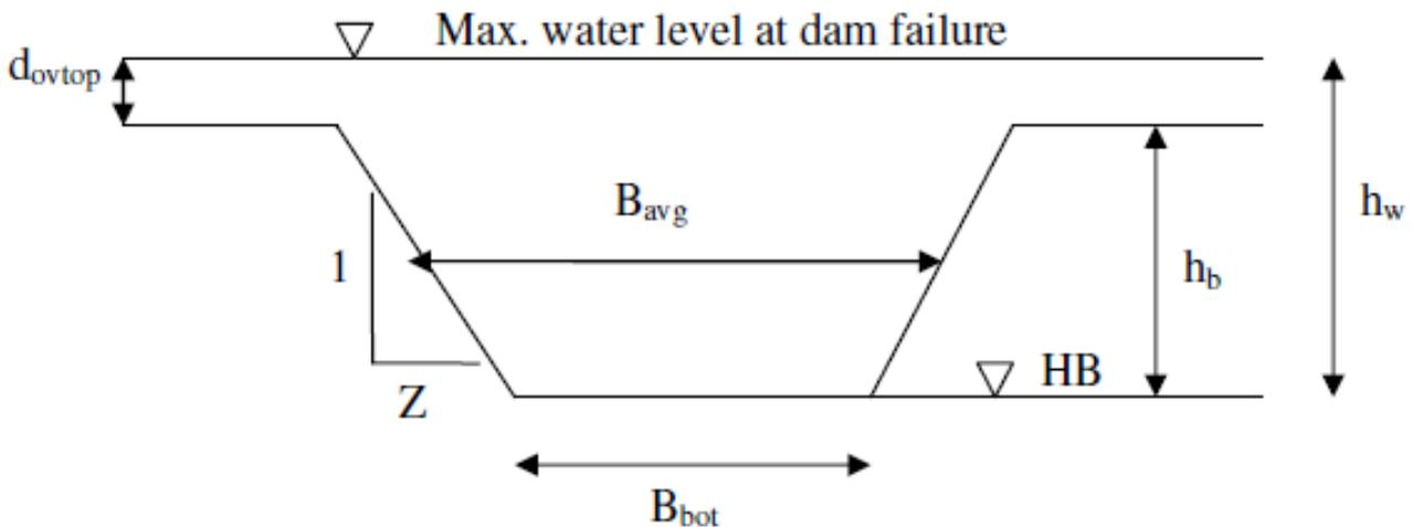
Fig. 2: Parameters of an idealized dam breach [18]
