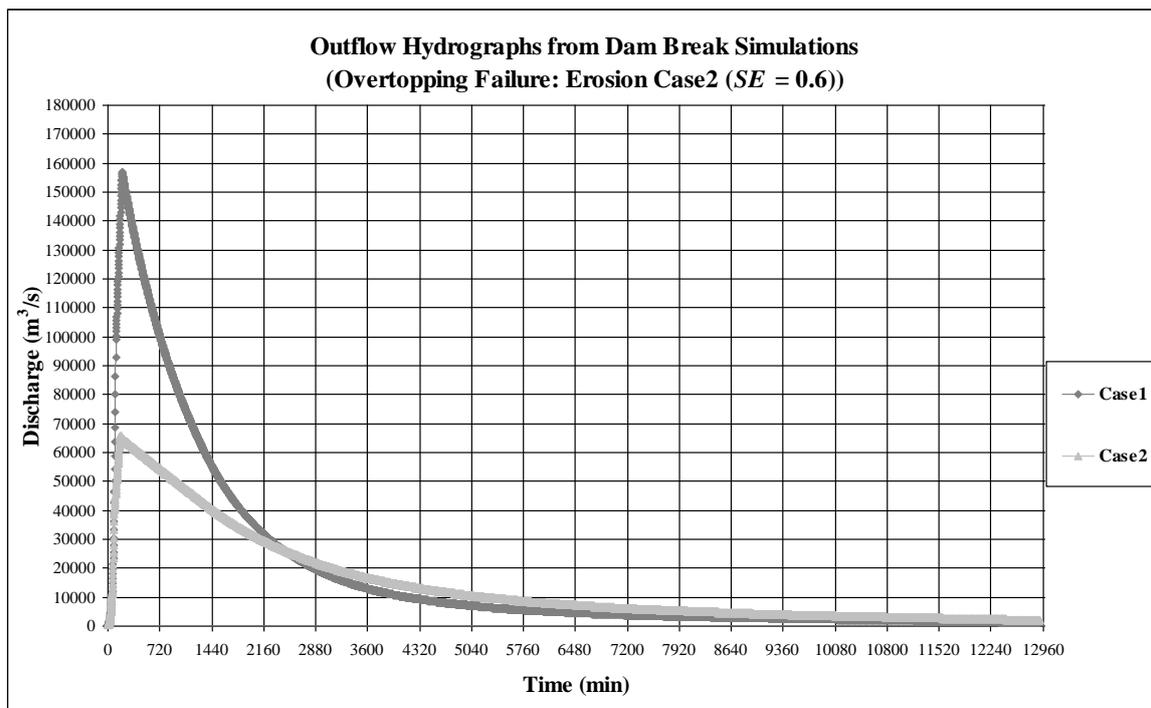
Fig. 5: Outflow hydrographs from dam break simulations (Erosion case2:  $SE = 0.6$ )
