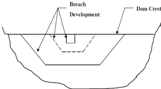
Fig. 3: Linear development of the breach [18]
