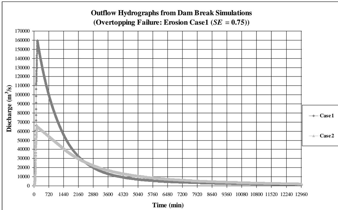
Fig. 4: Outflow hydrographs from dam break simulations (Erosion case1:  $SE = 0.75$ )
