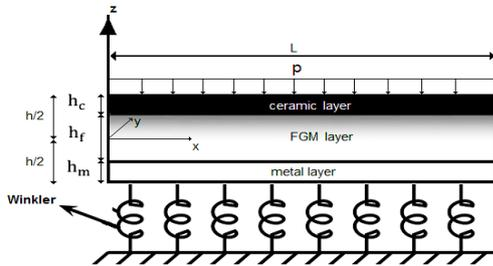
Fig. 1. Geometry and coordinates of sandwich beam resting on Winkler foundation.
