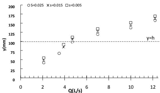
Fig 5-a: brushes effect on increasing channel depth on different slopes and charges -first arrangement
