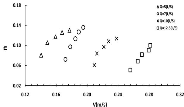
Fig 10: the Manning coefficient variations with velocity for the second arrangement
