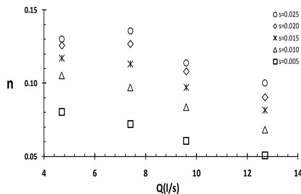
Fig 12: the Manning coefficient variations with discharge and slop for the second arrangement
