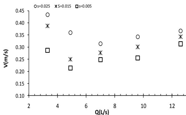
Fig 6-c: the brush Impact in reducing the channel mean velocity on different slopes and charges - third arrangement
