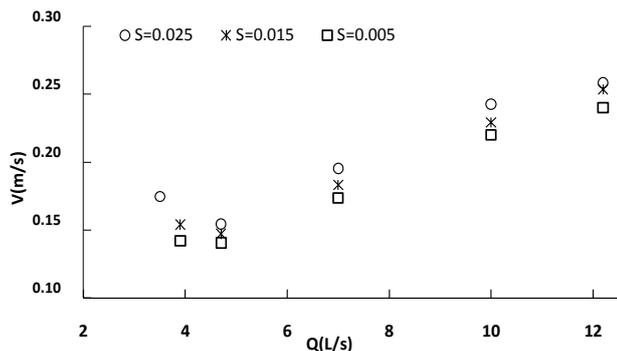
Fig 6-a: the brush Impact in reducing the channel mean velocity on different slopes and charges - first arrangement
