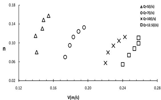
Fig 9: the Manning coefficient variations with velocity for the first arrangement
