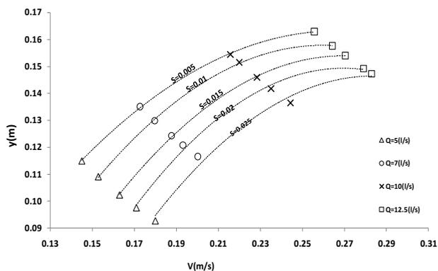
Fig 8: variations in mean velocity and the depth in submergence condition for the second arrangement
