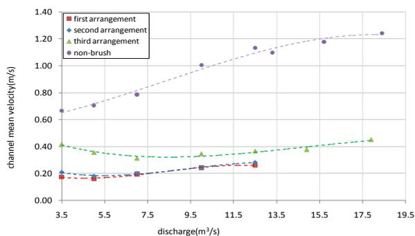
Fig 6-d: the comparison of mean velocity in three arrangements and also in the non-brush channel on 0.025 slope
