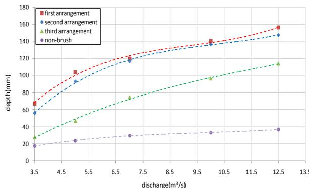
Fig 5-d: the comparison of water depth in three arrangements and also in the non-brush channel on 0.025 slopes
