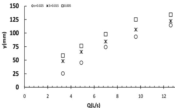
Fig 5-c: brushes effect on increasing channel depth on different slopes and charges - third arrangement
