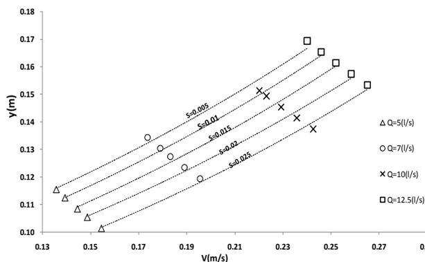
Fig 7: variations in mean velocity and the depth in submergence condition for the first arrangement
