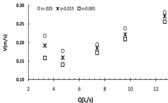
Fig 6-b: the brush Impact in reducing the channel mean velocity on different slopes and charges - second arrangement
