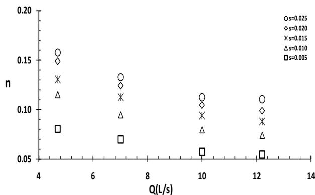
Fig 11: the Manning coefficient variations with discharge and slop for the first arrangement
